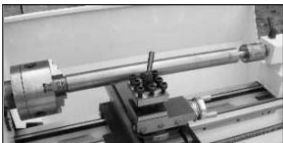
Figure-36 checking headstock and tailstock alignment
