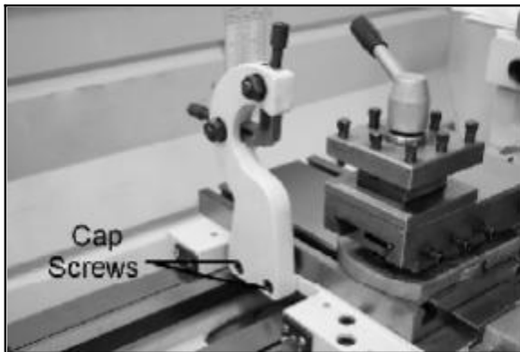
Figure-6 Follow rest installed
